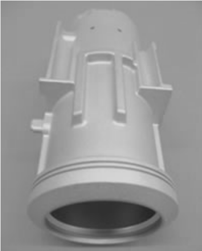
Aluminum housing plated 0.002 thick after finishing
