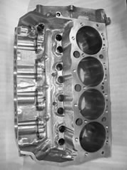
Cylinder Bores of large aluminum billet engine block plated with 0.004 thick NiCom after diamond plateau honing.
