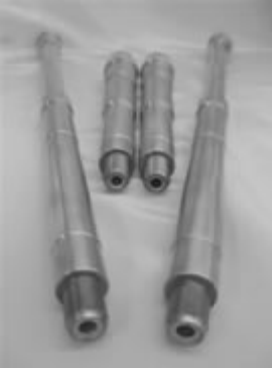
Bore/rifling of gun barrels electropolished and chrome plated 0.0004 thick chromium.
