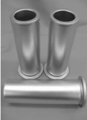
Pistons chrome plated 0.006 thick before grinding.
